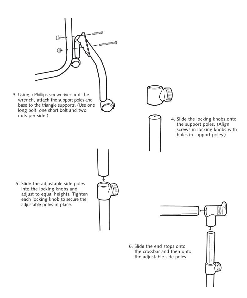
Now that your stand is complete, attach the pocket chart hangers by pressing each hanger opening onto the crossbar until the inner "ring" is resting on the crossbar.
