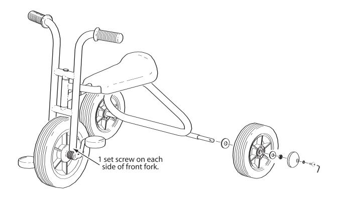
Before children ride their new vehicle, have an adult use the enclosed tools to tighten all preassembled hardware. Please refer to the above illustration to help you locate the set screws that require tightening. Once you have completed this step, the vehicle will be ready for use! To maximize safety, check the screws regularly, and tighten as necessary.
